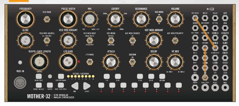
Kick sound comes from LFO being pushed into audible frequencies by the Envelope Generator. LFO RATE, along with ATTACK, DECAY, and SUSTAIN values can be altered to create kick drum variations.
