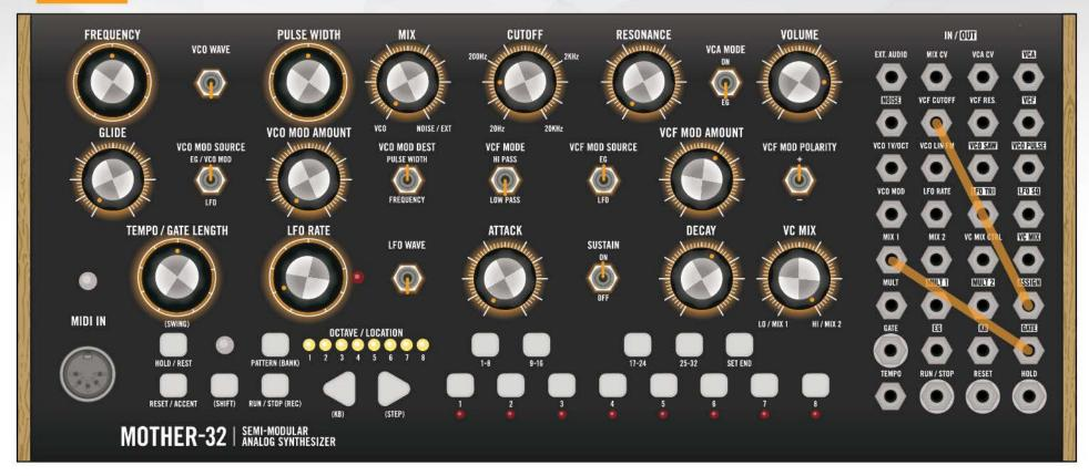
The ASSIGN output is changed to 8: STEP RANDOM, which creates a random CV for each step, making the Filter Cutoff move a random amount each quarter note.
