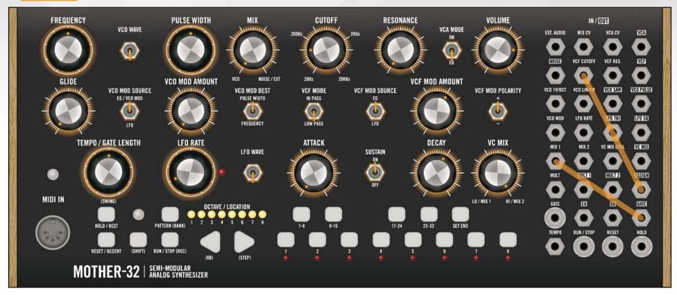
The ASSIGN (Assignable CV) output (set to 2: CLOCK) is connected to the VC MIX 1 input. The VC MIX output is connected to VCF CUTOFF which gets a CV pulse on every quarter note.
