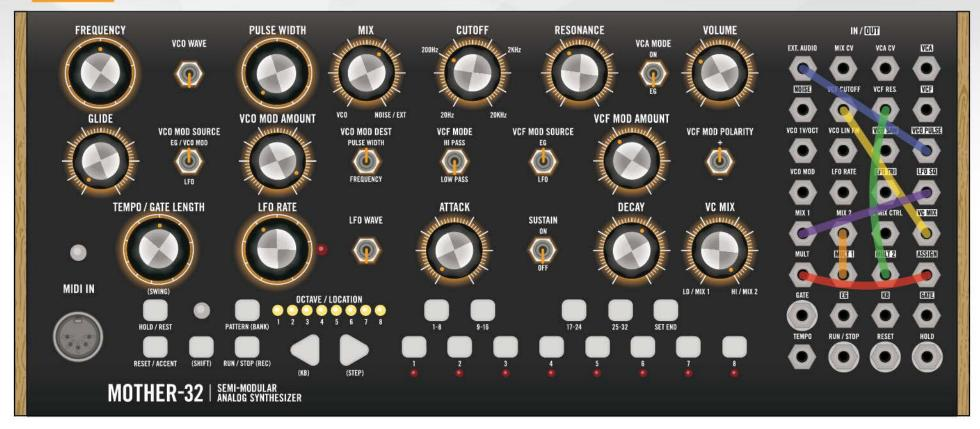
The ASSIGN output (set to 1: ACCENT) allows a choice of which sequence steps send higher voltage to the MULT. MULT 1 mixes with the LFO SQ to mod VCF CUTOFF. MULT 2 mods the VCF RESONANCE. LFO TRI sweeps the VC MIX between ACCENT and LFO SQ.
