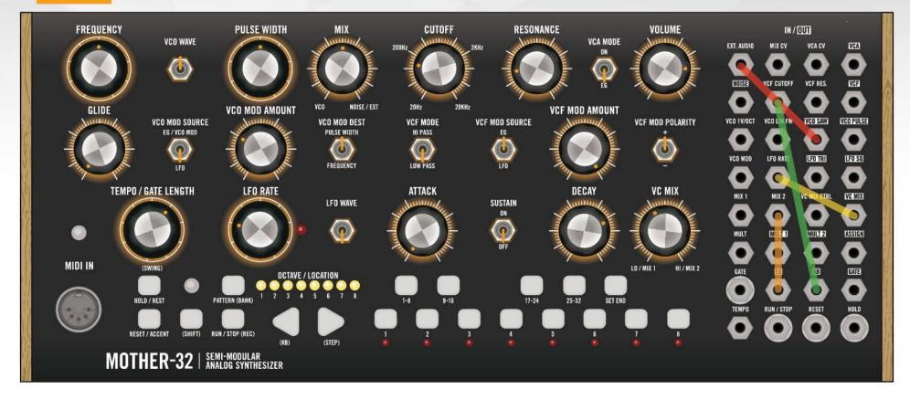
VCO SAW is connected to the EXT. AUDIO input so that both PULSE and SAW waves can be heard and blended via the MIX knob. VC MIX has been inserted between EG (Envelope Generator) and LFO RATE to allow you to dial in the amount of envelope modulation of the LFO RATE (which is creating Pulse Width Modulation) via the CV MIX knob. This makes for a more interesting Pulse Width sound.
