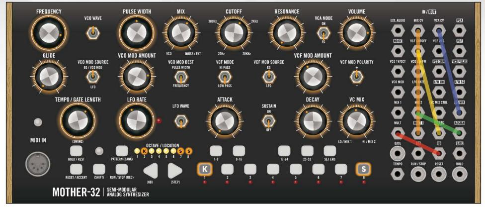
Connecting the ASSIGN output (set to 8: STEP RANDOM) to the CV MIX 2 input, and then the CV MIX output to the VCA CV input creates random rhythmic volume variations. The depth of the volume variations is set via the VC MIX knob.
