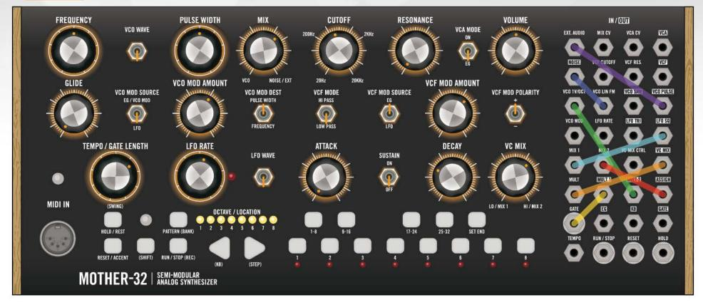
The ASSIGN output (set to 3: CLOCK/2) is sending voltage every other beat to MIX 2, while MIX 1 is getting LFO SQ. The VC MIX output is split with MULT 1 going to the GATE and MULT 2 going to the VCO's pitch.
