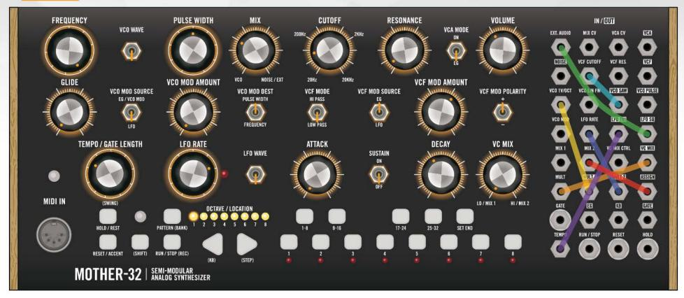
The ASSIGN output (set to 8: RANDOM) sends a random voltage each step to MIX 2, allowing the VC MIX knob to set the depth of randomness to both the LFO RATE and the sequence's TEMPO, which can go from plain to insane.
