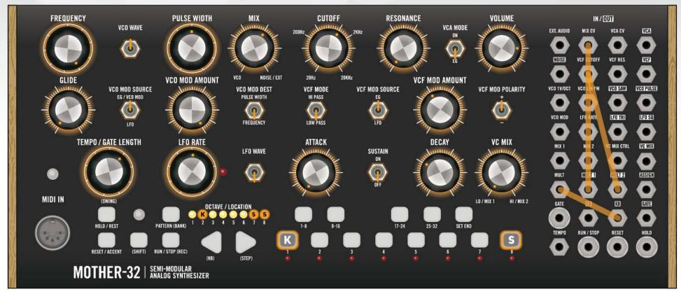
KB (Keyboard Tracking) is sent to MULT, which splits the CV into MULT 1 and MULT 2 outputs. One of them goes to the MIX CV input, swinging the mix between the PULSE VCO and NOISE. The other CV goes to VCF CUTOFF, making the sound brighter the higher you play on the keyboard.
