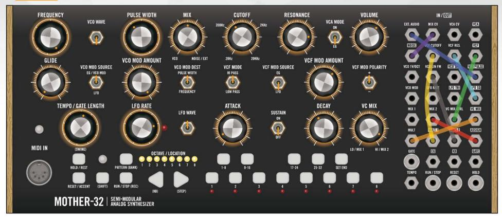
The ASSIGN output (set to 7: STEP TRIANGLE) goes to the CV MIX 2 input, and then the CV MIX output is sent to MULT, which splits the CV into MULT 1 and MULT 2 outputs. One goes to VCF Cutoff, the other to VCO LIN FM. LFO SQUARE mods RESONANCE, and NOISE mods the MIX.
