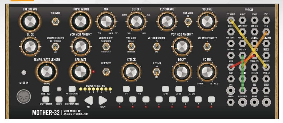
Mixing the LFO and VCO SAW together allows for more kick variations. Use the VC MIX knob to blend to taste.
